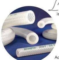
ow volatile grade, platinum-cured silicone hose is clean-room produced for critical pharmaceutical, biopharm, cosmetic and food applications. Polyester yarn braiding inside the wall enhances pressure capabilities. AdvantaSil APSH has undergone extensive physical, chemical and biological testing and meets USP Class VI, FDA CFR 177.2600, ISO 10993, European Pharmacopoeia 3.1.9 and 3-A standards.
