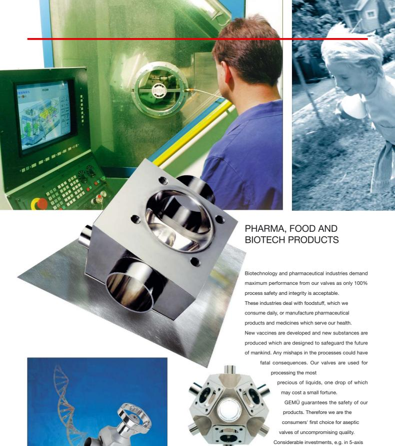
simultaneous CNC machines with CAD connection, were necessary to achieve such a performance capability. These machines produce GEMÜ M600 multi-port valves where all the valve weirs and cross connections are integrated "into one component".
